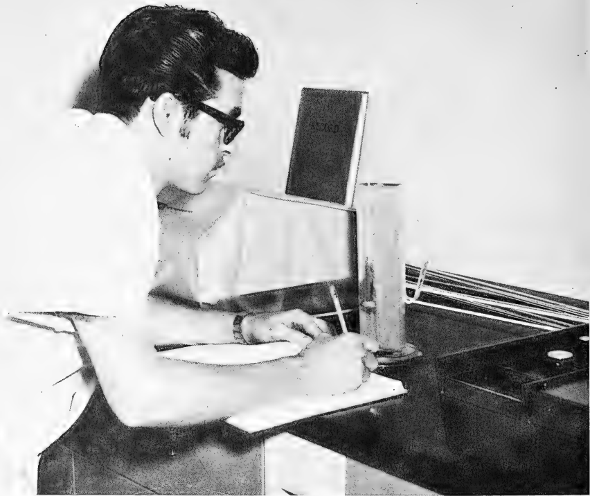
Figure 9.--Technician using a hydrometer to measure salinity of a sample of San Francisco Bay water.
